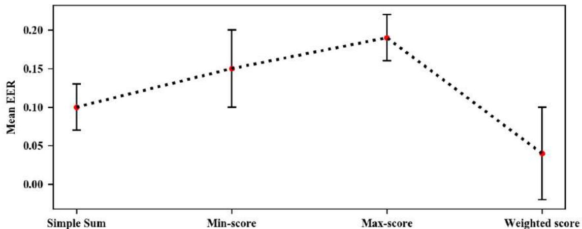
**Figure 9. Mean EER from score fusion methods for swipe gestures and signature combination using the commercial signature verification system from scenario 1 of Session 1**
